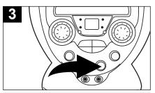
Adjust the AVC control as described below. Slide the CDG/CAMERA switch (rear of the unit) to the CDG position to see the CD+G lyrics on the external TV.
